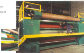
4,5 m. wide beltbonder under construction
