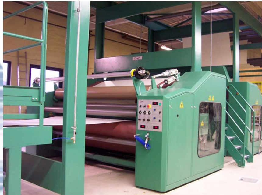
2 x LFC 141/2750 for laminating and for thermobonding
