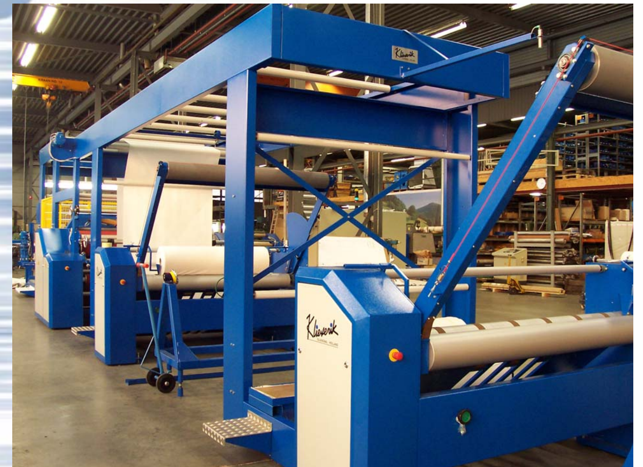
A combination of two Big Batch Un-winders and high in-feed with Laminating Calender LFC 131/2000, an accumulator-40M and contact winding device.
