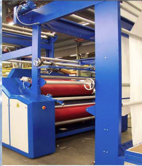
High in-feed and Laminating Calender
