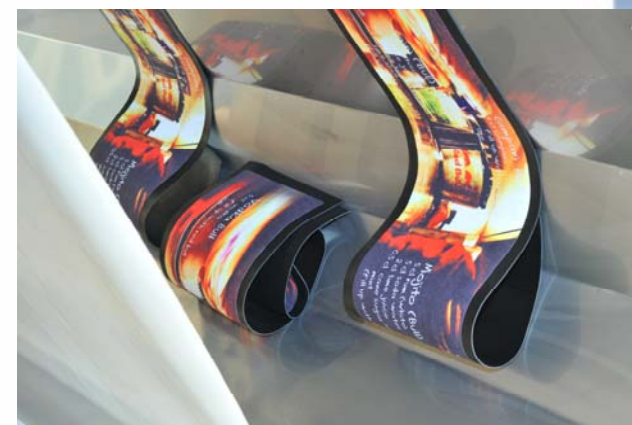
Transportation of printed pieces to J-box. The single items are transported automatically through the calendar without the need to use "sticky" paper.
